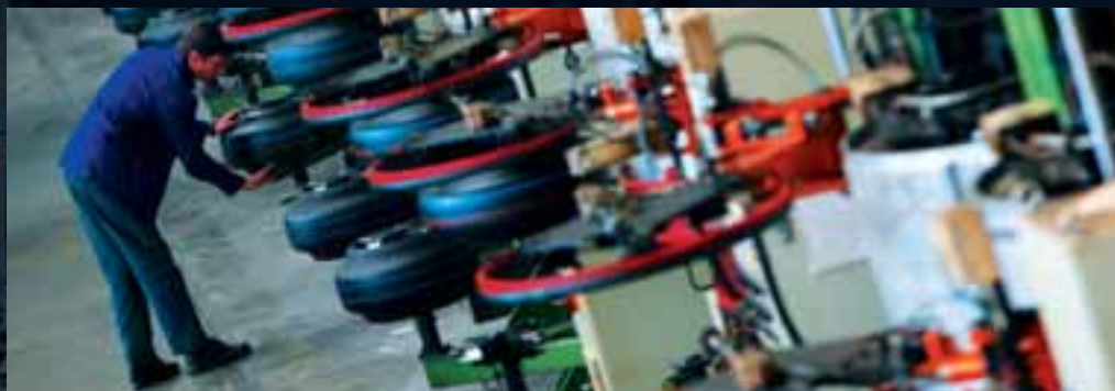
Tyres after vulcanization at Moscow Tyre Plant
